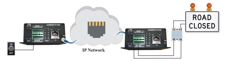
The above example shows two HARMONY IP I/O8 devices linked together using an Ethernet connection. A switch on the IP I/O8 device on the left is used to remotely turn the ROAD CLOSED flashers on or off via the IP I/O8 device on the right.
