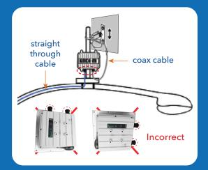
NON-INTEGRATED BROADBAND RADIO WITH PANEL ANTENNA
